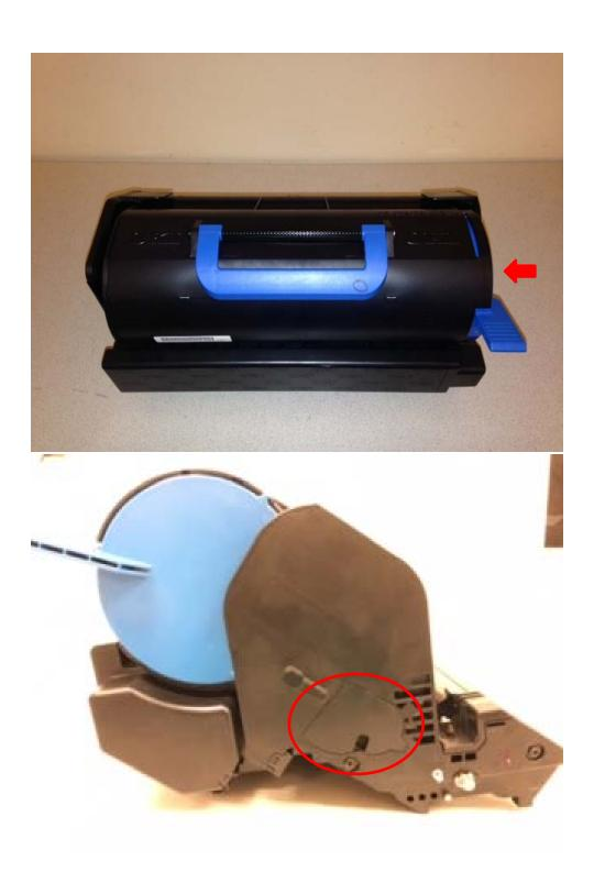
With the print cartridge sitting on the flat surface look into the small window in the access panel. Move the blue lock lever to the down / unlocked position. You should see the black lever behind the access panel blocking the small window (see red circles below).
