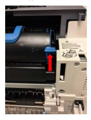
Ensure blue lever is in up position, then close the front cover and see if the 543 Toner Sensor Error clears. If the error clears, there is no need to read beyond this point. Procedure completed.
