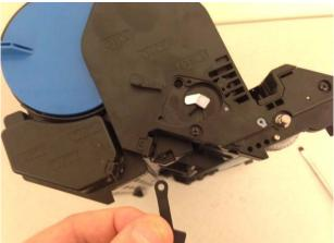
Now that the black lever has been removed replace the access cover. Line up the three studs on the back side of the of the access cover with the corresponding holes in the print cartridge. Then press the access cover into place with your finger.
