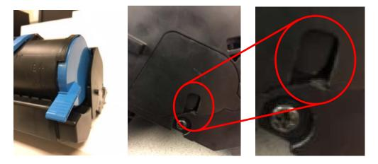
Now move the blue lock lever in the up / locked position. You should not see the black lever behind the access panel blocking the small window (see red circle below).
