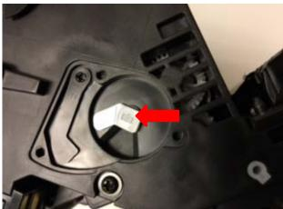
Once the access panel has been lifted off the print cartridge you can remove the malfunctioning black lever (see red arrow below).
